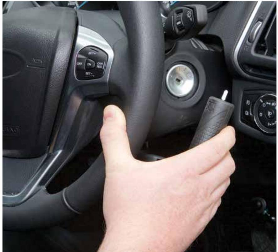
A push/pull device is a good option if you find it difficult to use standard foot pedals to accelerate and brake. You just pull the control towards you to accelerate, then push away to brake. Push/pull devices are designed for use with automatic gearboxes only.
